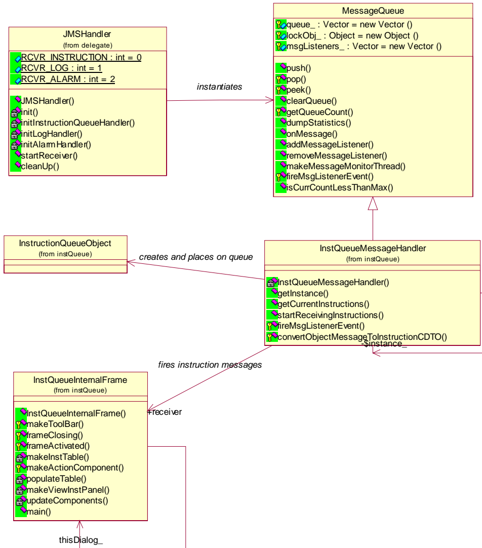
Figure 14: Message Queue Class Diagram
